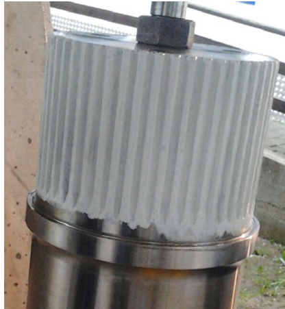
Illustration 4: Correctly lubricated splined shaft connection
