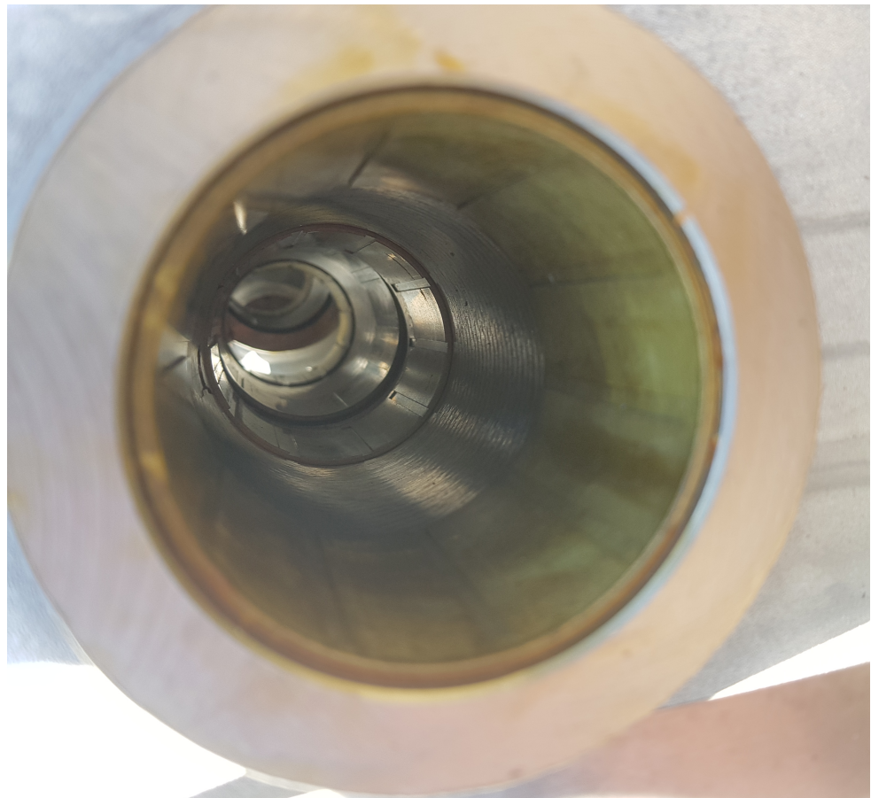
Illustration 3: Corrosion layer or protective lubricating film layer removed without residue
