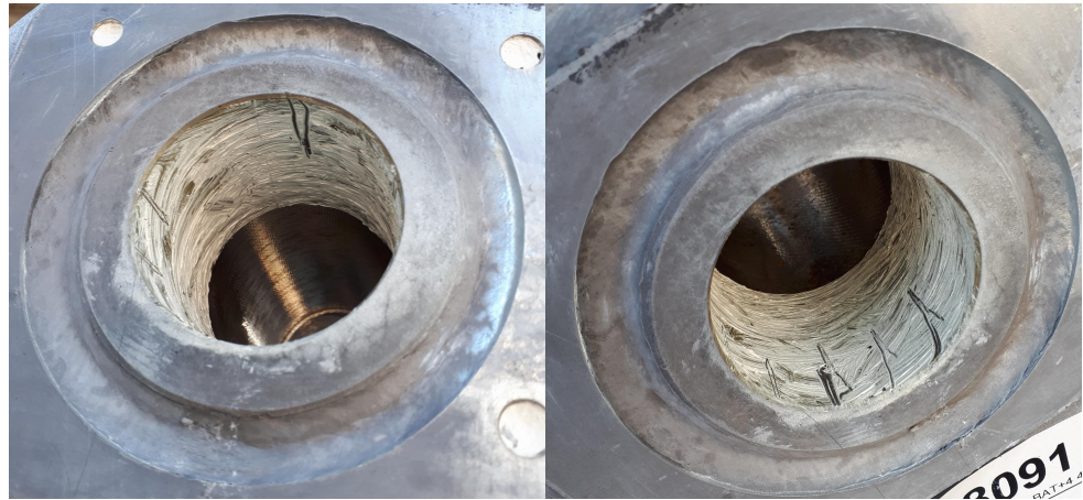
Illustration 1: Apply sufficient lubricant for basic corrosion protection
