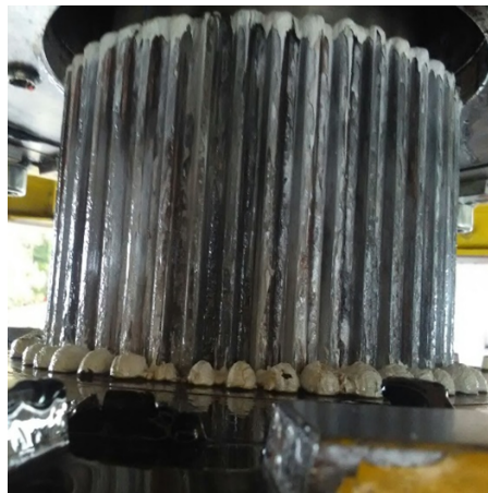
Illustration 5: Incorrectly lubricated splined shaft connection
