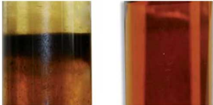
Illustration 1: Comparison between non-miscible and miscible oils
