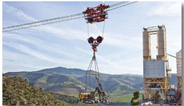
*Our slack carriers support the haulage and hoisting lines and provide fast traverse carriage speed by an absolutely smooth service and low sheave and rope wear. This means no system downtime for repairs or maintenance.*
